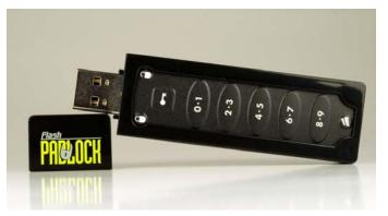
*Flash Padlock* is a *self-secured*, *platform independent* USB Flash Drive with a *hardware-authentication mechanism*. When locked, a Flash Padlock is invisible to its host; when unlocked, it acts as a standard USB Flash drive.
